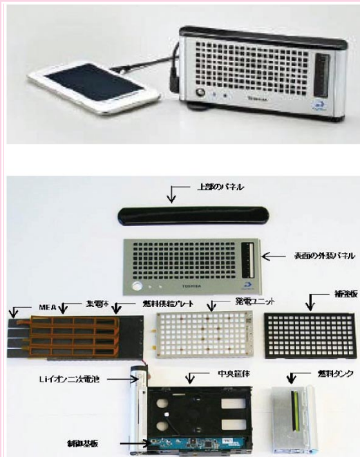
Figure 12 Component parts of Dynario
