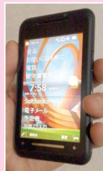
Figure 13 Built-in type DMFC prototype for a smart-phone
