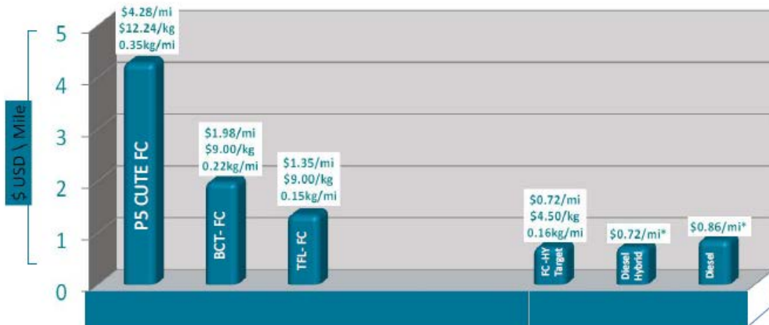
Fig. 5. Fuel costs for fuel cell and diesel/diesel-hybrid transit buses. To become competitive with conventional transit buses will require improvements in fuel cell efficiency and hybridization strategies, and a considerable reduction in the cost of H 2 .
