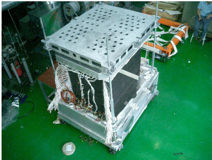
Figure 7. 75 kW test stack for the development of the 250 kW system at KEPCO
