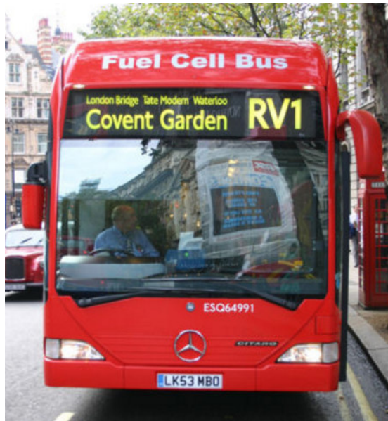
FIGURE 179 London bus on the RV1 line, powered by Ballard FC Velocity-HD6 PEMFC modules delivering 150 kW 6
