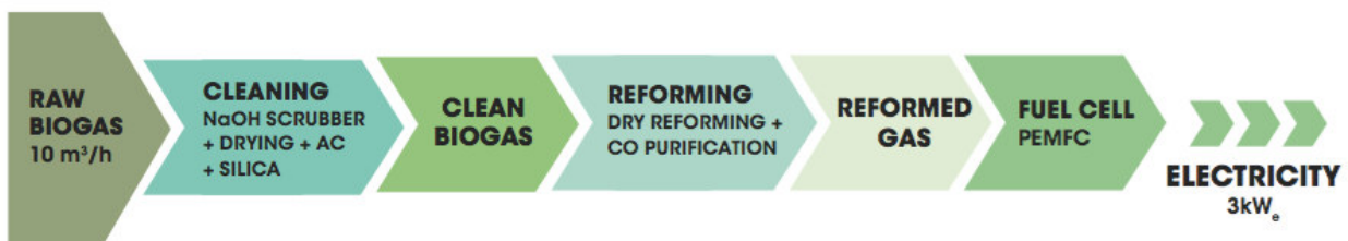
FIGURE 250 Flowchart of the PEMFC integrated pilot system in Murcia
