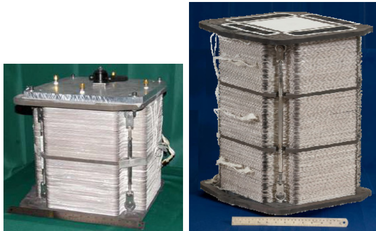
Figure 23. 11 kW stack (characteristics: 64-cells, 550 cm 2 active area 0.313 W/cm 2 peak power density at design load, 61.5 fuel utilisation, from 10 to 18% air utilisation, 200 A stack current, 730-750 °C cathode outlet temperature) and 3 stack blocks of 10 kW into 30 kW stack module. [sources: Proceedings of Fuel Cell Seminar 2011, Proceedings of SECA Workshop 2012]
