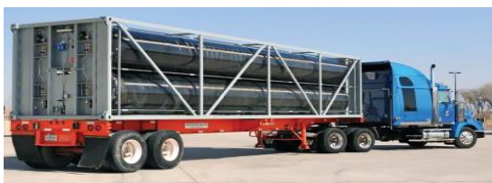
Hexagon Lincoln's 3,600 psi TITAN™ Tank and Frame System
